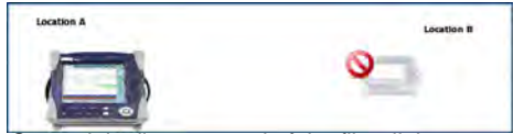
One unit is disconnected of the fiber link, or there is a break
