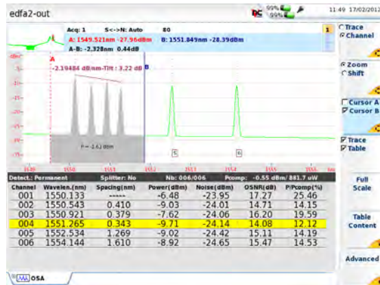
Figure 145 Display of total power, gain tilt and slope of the gain between the cursors
