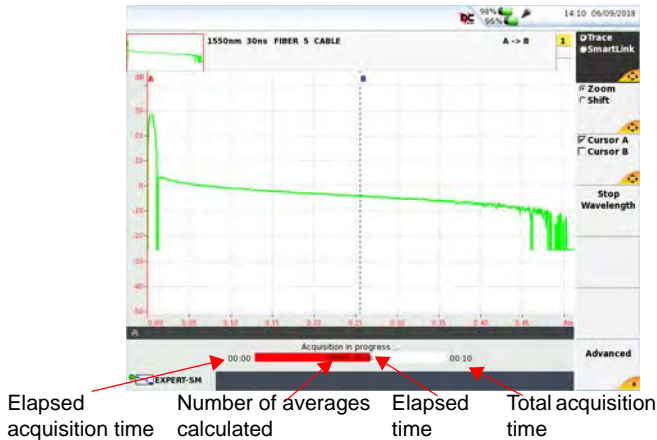
Figure 31 Acquisition in progress with Expert OTDR
