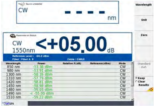
Figure 111 Results and commands of the power meter
