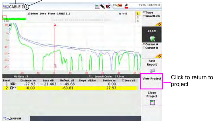
Figure 63 Trace from fiber selected in project Name of the label Number of the fiber tested
