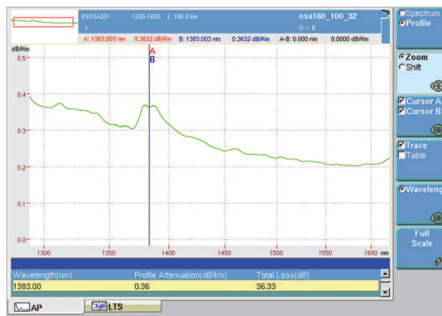
Figure 6. OTDR measurement at 1383 nm with VIAVI OTDR
