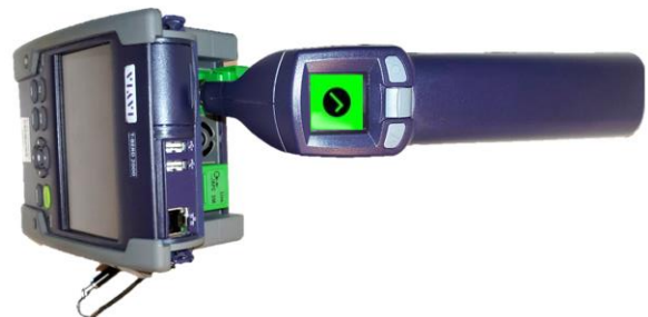
Figure 3: OTDR Port Inspection
