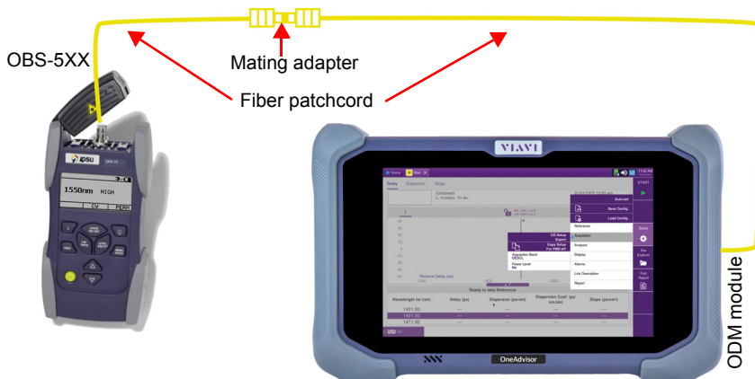
Figure 24 Reference measurement setup with an OBS-5XX
